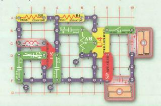
Adjusting the variable capacitor changes the range of frequency that you are listening to. The high frequency IC amplifies and decodes the modulation into the original signal (voice or music). This is amplified by the power amplifier IC. Varying the adjustable resistor makes the sound louder or softer.
